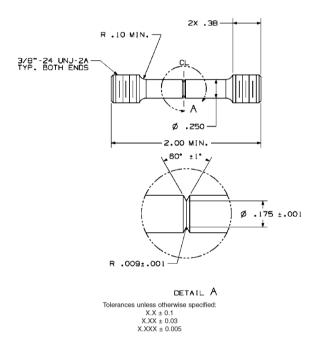
3. The tests are to be performed in accordance with the **EN 2832-93** or **ASTM F519-18** and the below requirements and test conditions:
